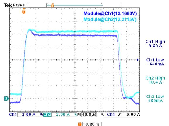
Fig. 4. Step-load response 0A/20A@2.5A/ $\mu\text{S}$
