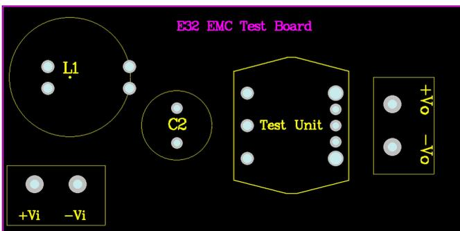
Fig.3 Top-side Layout of EMC Test Board
