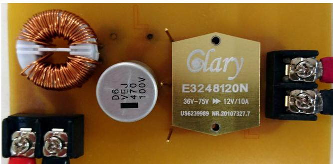
Fig.1 EMC Test Board with E32 Module
