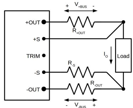
$$R_{-S} = \frac{(5V_{-BUS} + \frac{0.05I_o}{I_{RATED}})V_{RATED}}{V_o + V_{-BUS} + (\frac{I_o}{60I_{RATED}} - 1)V_{RATED}} - 3$$
