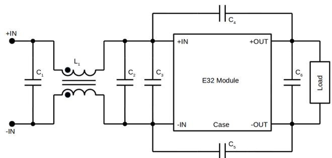
Fig.2 Circuit of EMC Test Board with E32 Module
