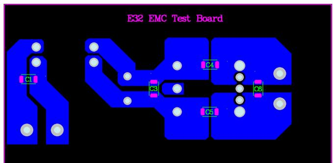
Fig.4 Bottom-side Layout of EMC Test Board
